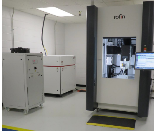
Rofin's UW1200 is offered in 5-axis or 3-axis versions with fiber or CO2 lasers.
