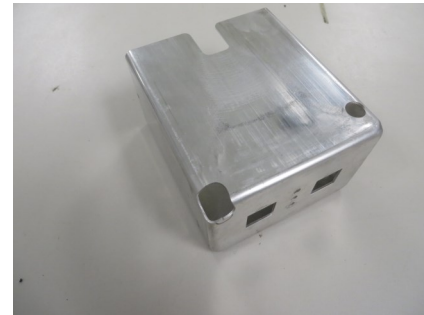
Hudson's runoff part required challenging flange, hole and slot cutting on all surfaces and across corners achieving accuracies of under \pm .005 ".
